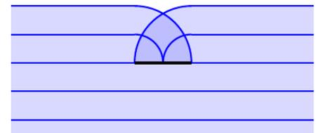
Figure 2: Diffraction around a narrow obstacle
