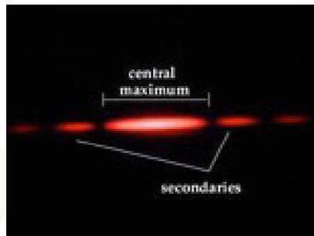
Figure 3: Interference Pattern of LASER Light
