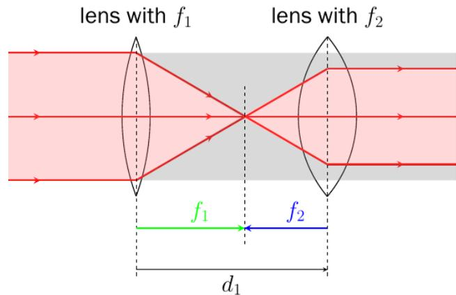
Figure 4: First Two Lenses of Rochester Cloak
