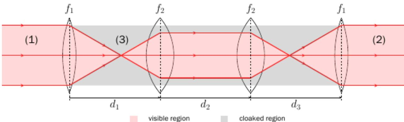
Figure 3: Ray Optics of a Rochester Cloak
