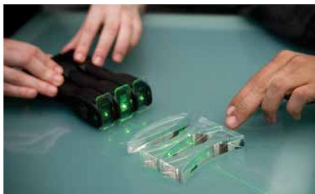
and refract. In addition, the suction mount can hold three lasers, which allows them to be positioned in parallel paths without having to hold them in place. Because the lenses are backed with a magnetic backing, I could then attach different lenses to the whiteboard in the path of the light to show how the different lens shapes bent the light into different patterns.
